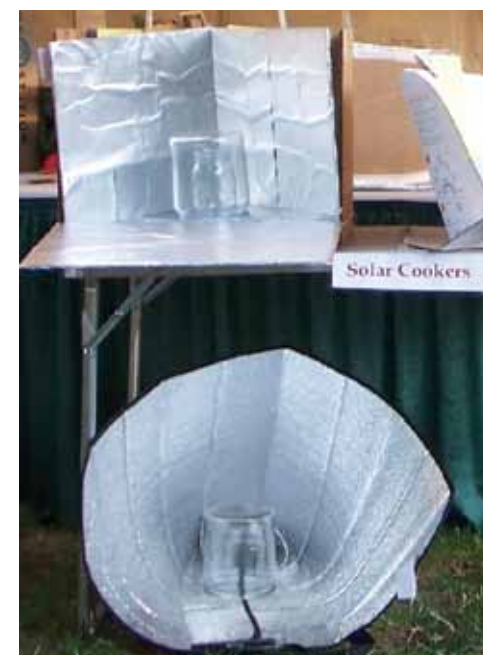
Solar cookers made from cardboard and aluminum foil and from a car window shade
